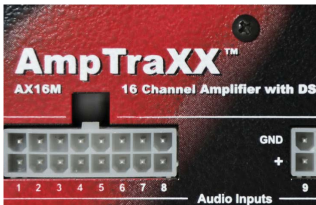
AmpTraXX is a DSP-enabled 16-channel ride vehicle amplifier
