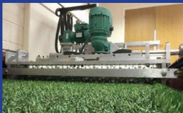
A great deal of compliance testing is called for to evaluate materials being supplied to sites to confirm that these match that original declared. Sports Labs provide testing to contractors looking to confirm compliance of materials such as shock pads and seam samples routinely.
