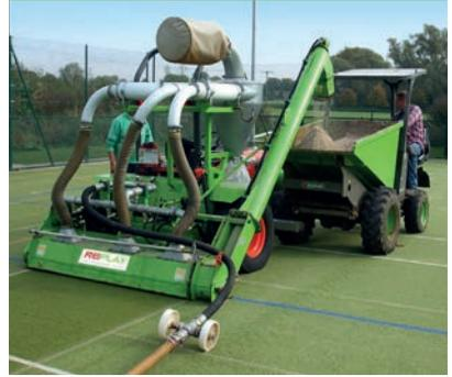
The unique **REPLAY REJUVENATION**® air extraction process will restore contaminated and compacted carpet to a clean 'as new' condition – extending the life of the facility at a much lower cost than replacement.
