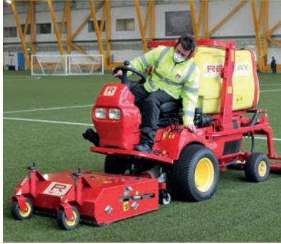
Our **REPLAY REVIVE**® multi-brush process penetrates the surface, decompacting and agitating the infill whilst removing dust, dirt and detritus leaving a cleaner and safer facility.
