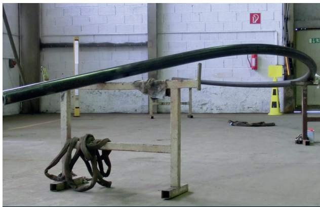
Track tubes bent by Maurer's XBEND machine
