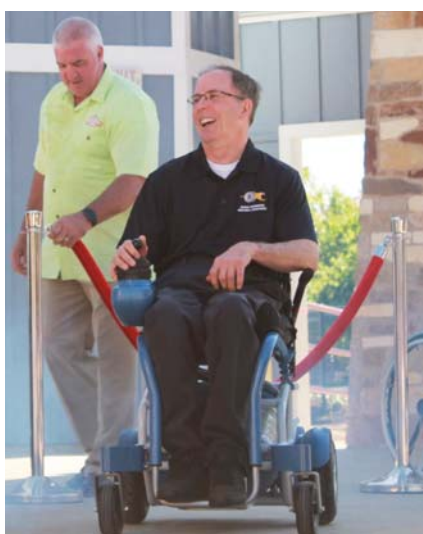
'PneuChair' can be operated using a joystick
