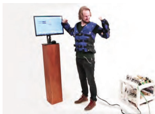
■ Inflatable compartments are used to simulate pressure
