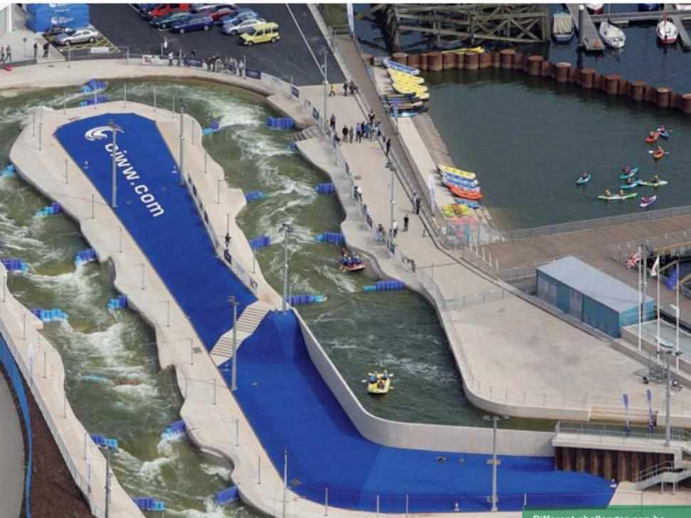
Different challenges can be created by moving the blue plastic barriers and adjusting the speed of the water being pumped around the course
